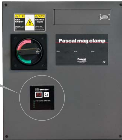
7-segment status indicator Built-in control box
