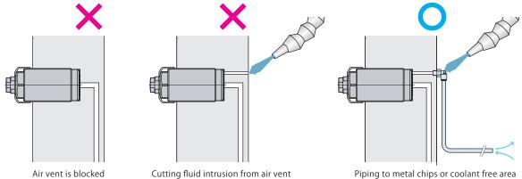
lacktriangle Air (oil free) must be fed through a 5  $\mu$  m filter that is connected to an air vent port for air cleaning. Perform air cleaning only when replacing workpiece. Plunger will rise during air cleaning.
