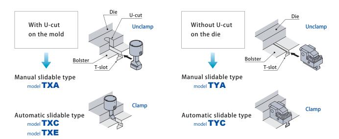
\* The unification of die thickness is conditions for the clamp use. If it is not unified, contact Pascal.
