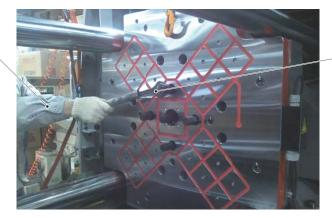
Poor workability and tool dropped easily in machine.
