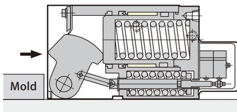
At time of unclamping, the lever is retracted back in the body and it does not interfere in loading/unloading the mold.
