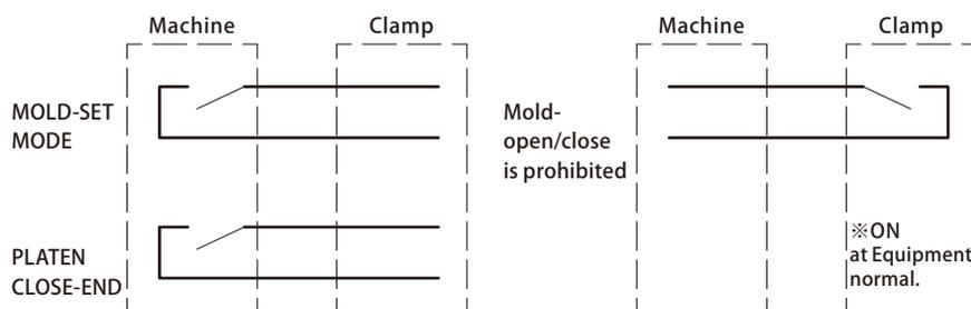
1. Signals to be output on normally open, zero-potential contacts.
