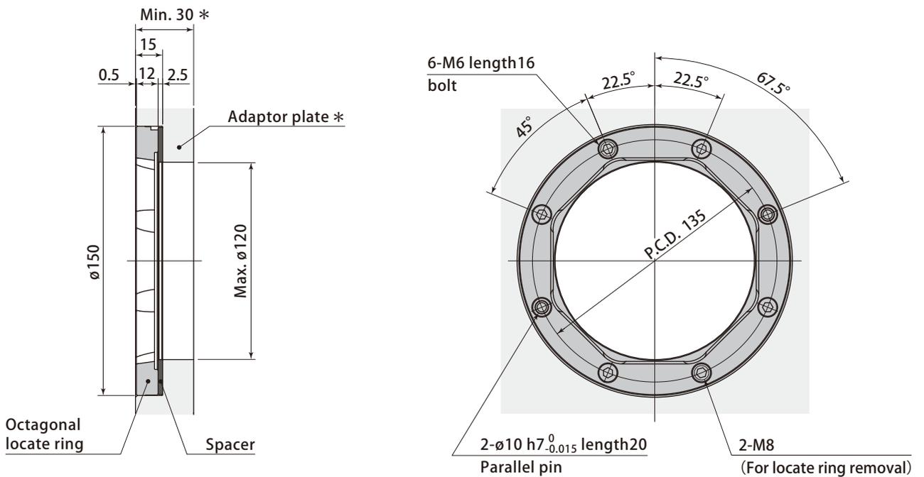
The adaptor plate thickness should be over 30mm when it is mounted on the plate.
