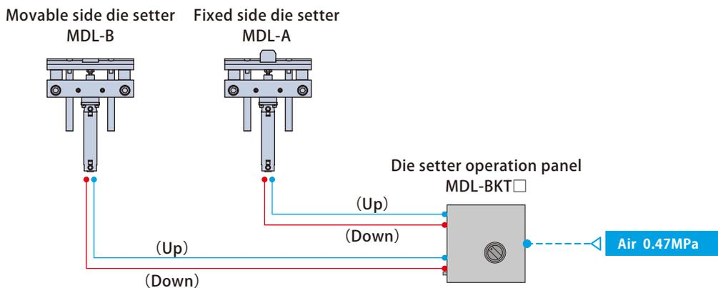
Die setter and clamp operation panel is used (in case it is incorporated in the control device)
