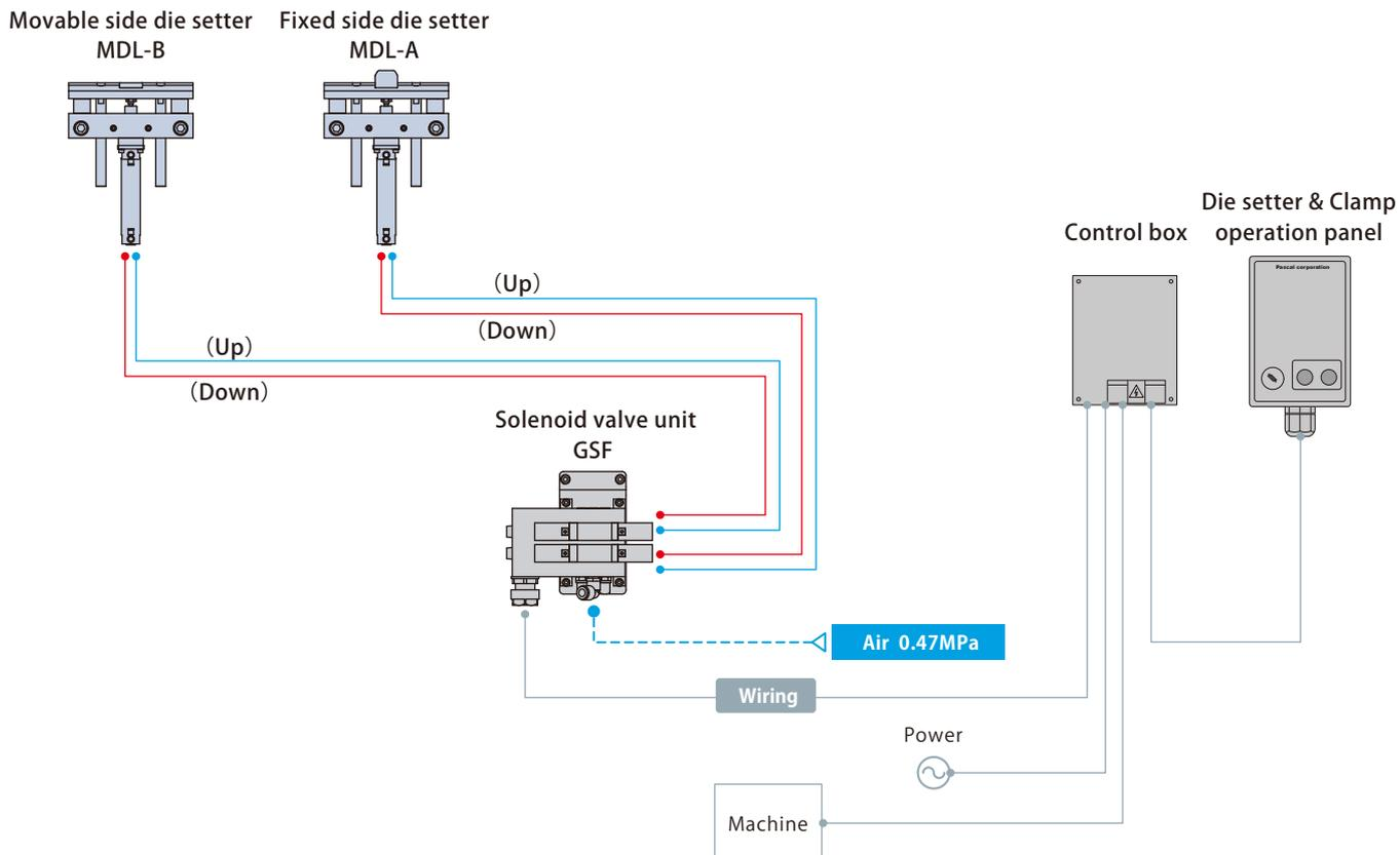
Die setting system MDL circuit
