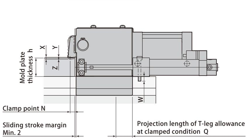
T-slot dimension and mold plate thickness
