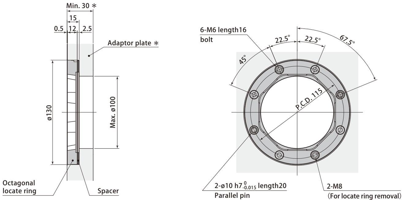
The adaptor plate thickness should be over 30mm when it is mounted on the plate.
