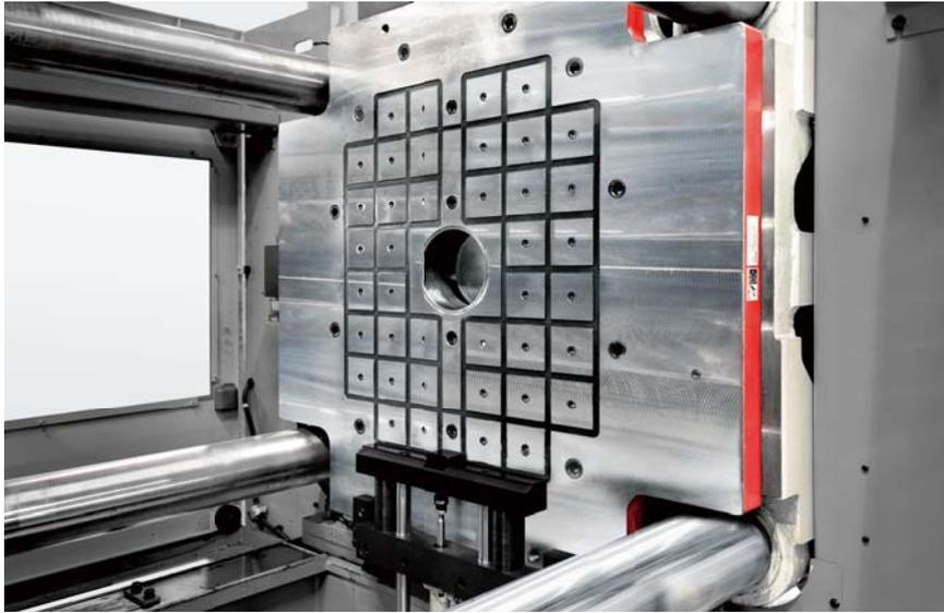
3,500kN (350ton) IMM vertical loading Die setting system & Mag clamp
