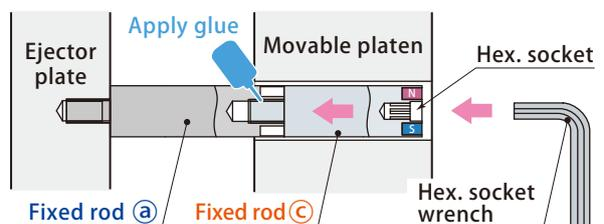
Applied for large sized IMM with the ejector stroke more than 300mm.
