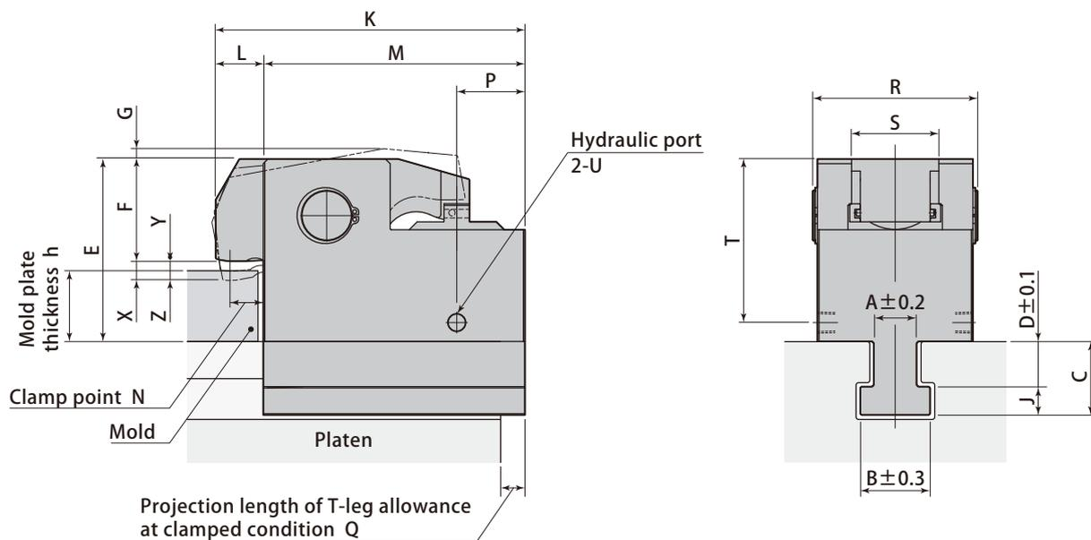
T-slot dimension and mold plate thickness
