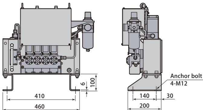
It is utilized to select the hydraulic clamp TKB and to supply the hydraulic pressure source from machine.
