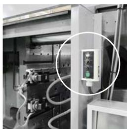
Compact design panel with L-shape mounting bracket enables installation near machine panel.
