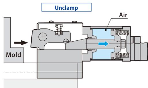
It slides automatically with air cylinder.
