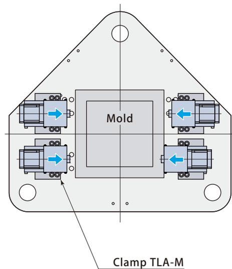
Air clamp, T-slot-less slidable type **TLA-M**
