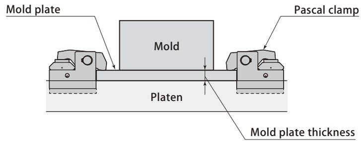
In case that the thickness of mold plate is not unified,
