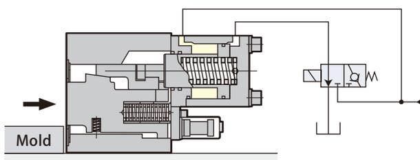
At time of unclamping, the lever is retracted back in the body and it does not interfere in loading/unloading the mold.
