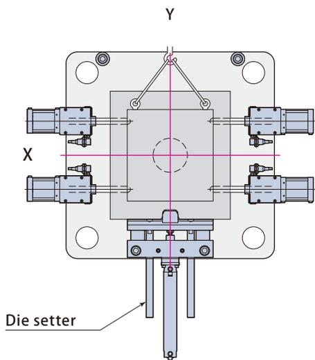
By placing the mold on the die setter, die setting is easy.
