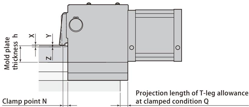
T-slot dimension and mold plate thickness
