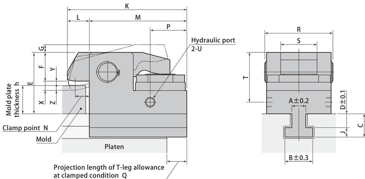
T-slot dimension and mold plate thickness
