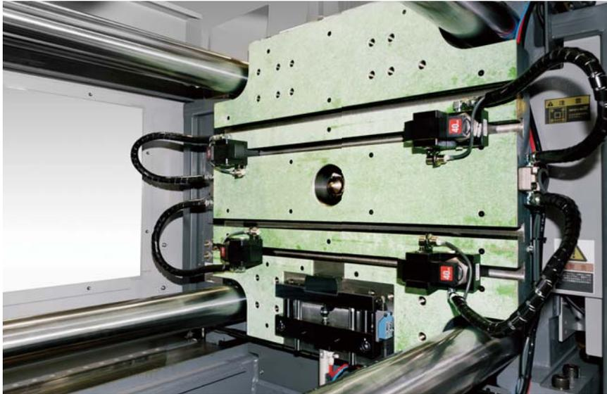
1,800kN (180ton) IMM vertical loading Die setting system & Hydraulic clamp, slidable type TYA040
