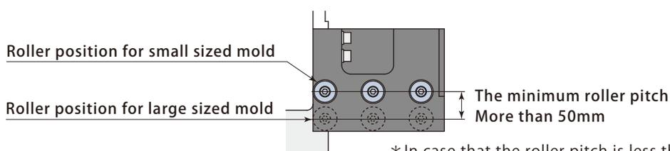
\*In case that the roller pitch is less than 50mm, contact Pascal for details.
