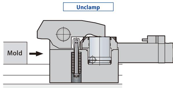
It slides automatically with an air cylinder.
