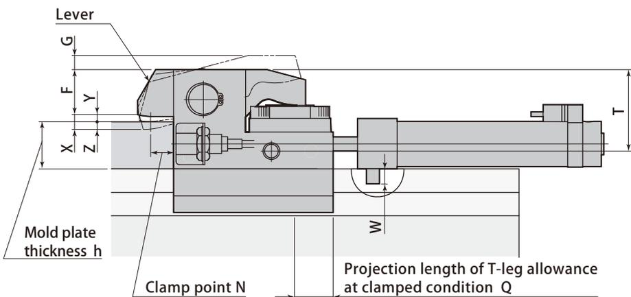
T-slot dimension and mold plate thickness
