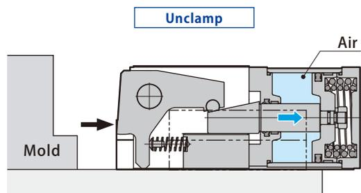
The clamp lever is **not retracted** back in the body at time of unclamping.
