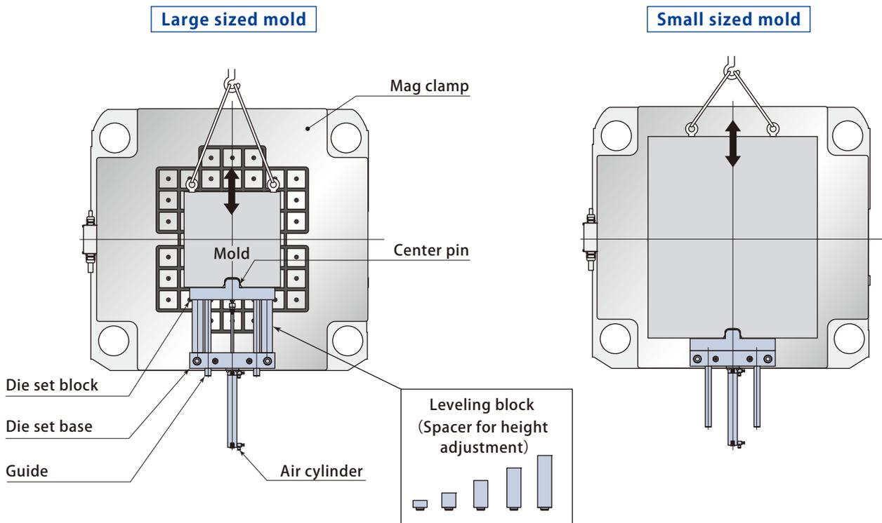
Die setting roller & Mag clamp (horizontal loading)
