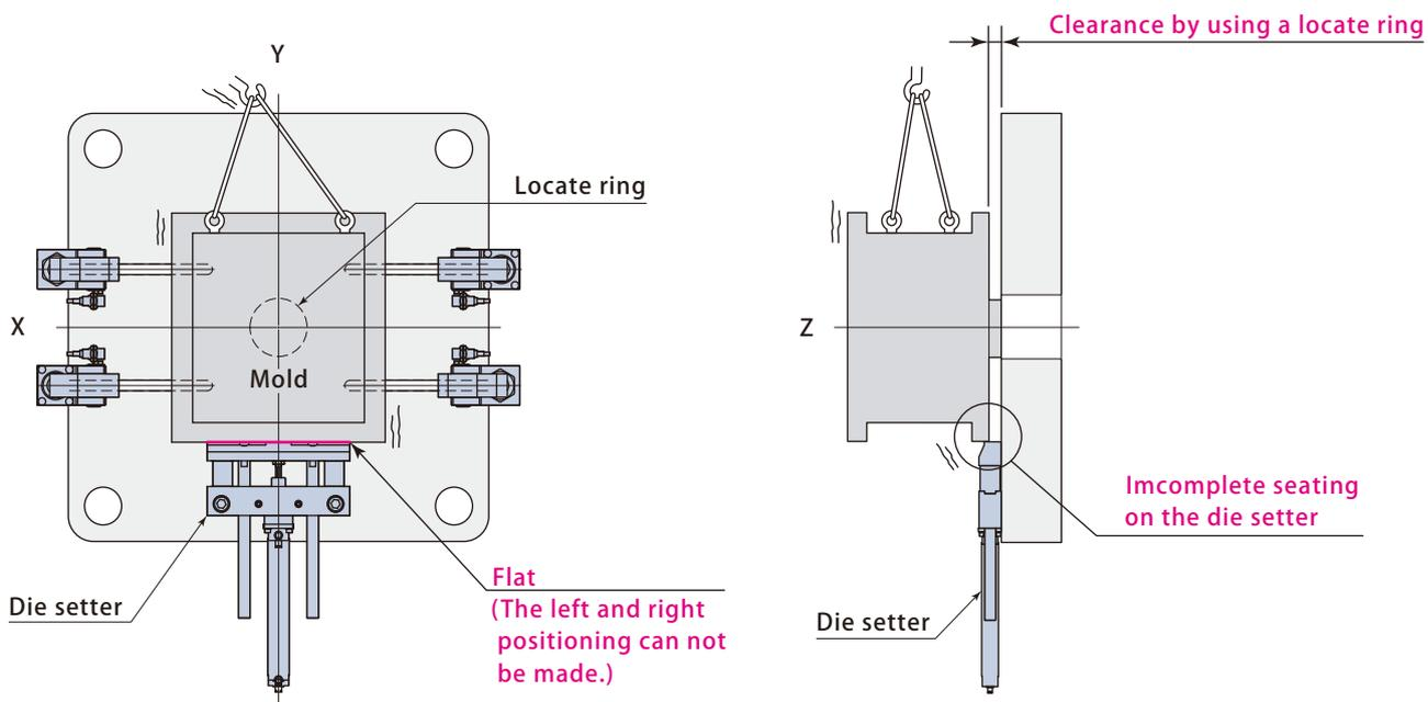
In case of using die setter for the mold with no U-cut, keep it out of the range of the mould mount area in advance not to interfere each other.
