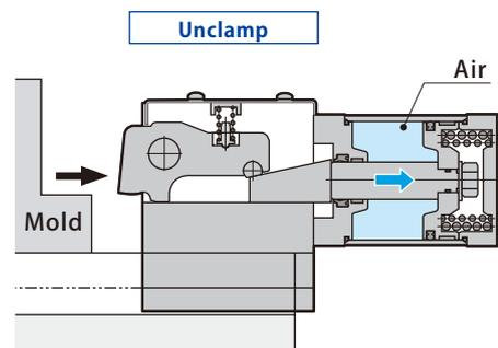
It is mounted on the T-slot and slidable by hand. The clamp lever is **not retracted** back in the body at time of unclamping.
