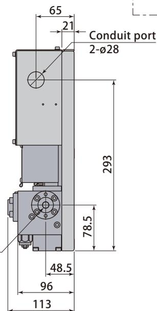
Non-leak valve unit VSE
