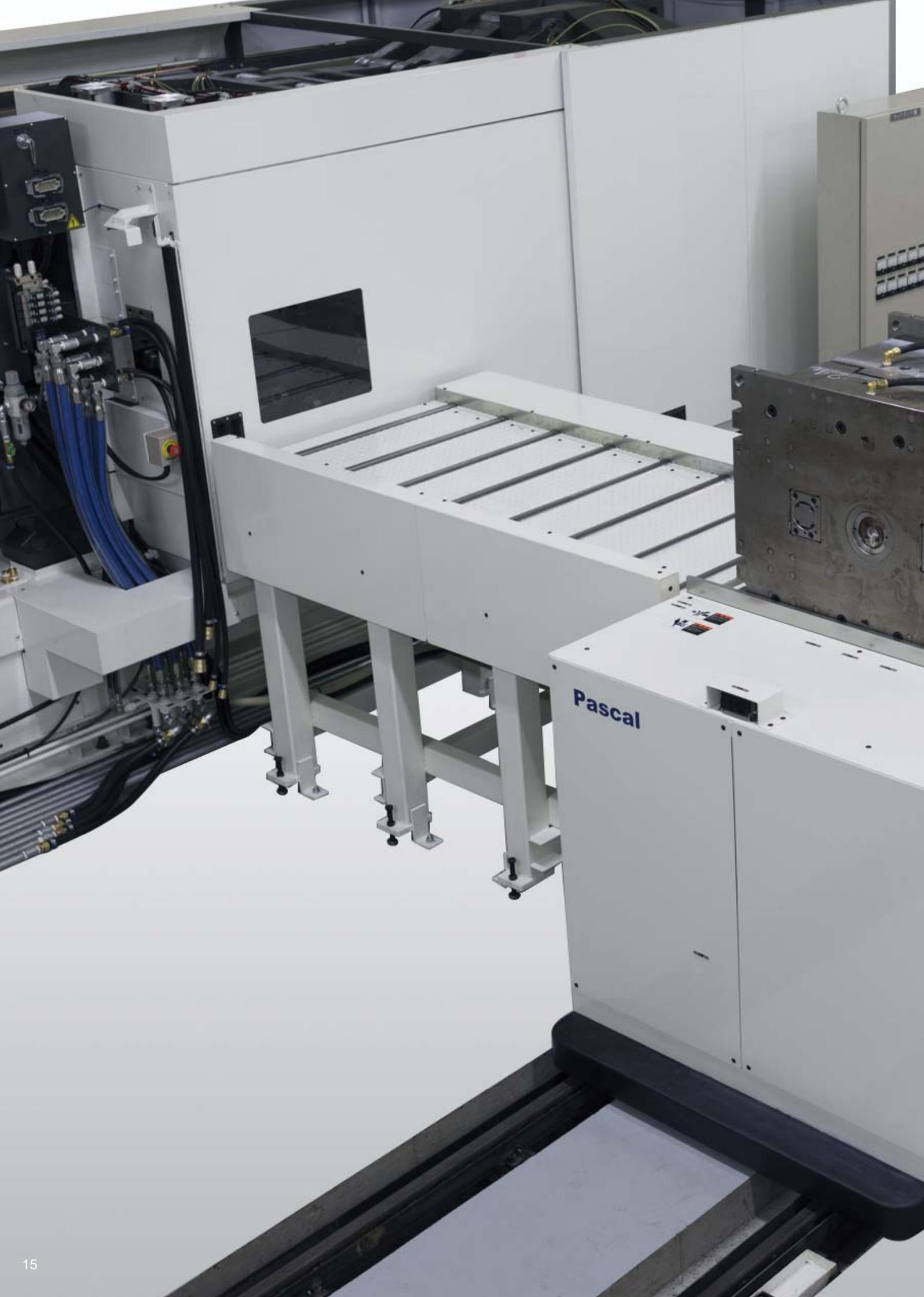
Air clamp, bolted type **TLA100** & Mold die changer
