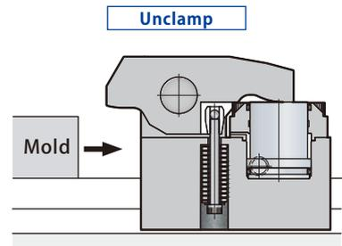
It is mounted on the T-slot and slid manually.
