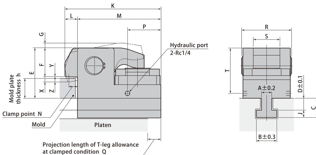
T-slot dimension and mold plate thickness
