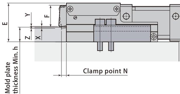
Air clamp, T-slot-less slidable type **TLA-M**
