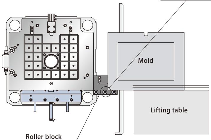
**No modification is required on mold.**
