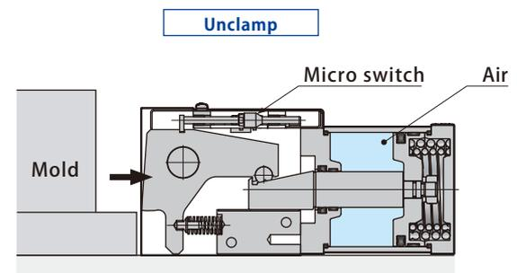
At time of unclamping, the lever is retracted back in the body and it does not interfere in loading/unloading the mold.
