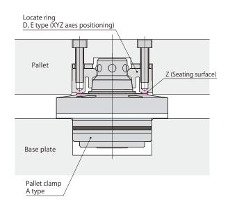
Since Z axis is positioned by 2 points of seating surface with no effect from pitch error, surface accuracy of pallet is sustained at high levels.
