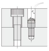
Chips accumulate and are trapped, becoming difficult to remove.
