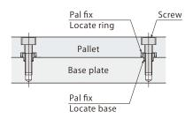
The diamond pin must be mounted perpendicularly toward round pin in addition to keeping the pitch accuracy between the two.
