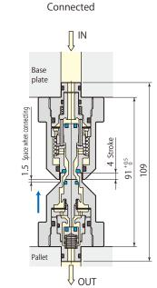
Perform installation with plug below so metal chips are less likely to adhere and air blowing can be performed properly.
