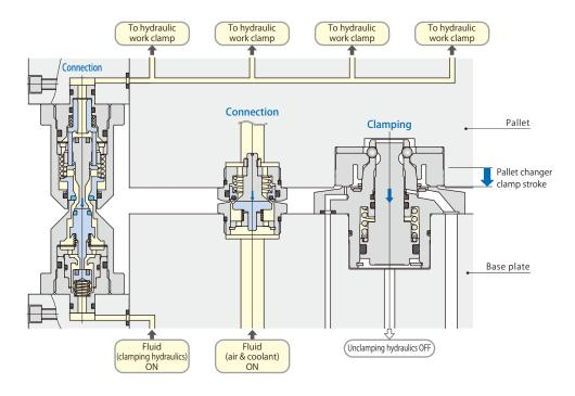
When clamping pallet, coupler connects due to clamp stroke of pallet changer, with hydraulics sustained.
