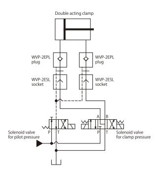
3 position, center tank-port solenoid valve should be used for clamp pressure circuit to avoid back pressure. A solenoid valve which switches to Tank port connection except supplying pressure to the circuit should be used.
