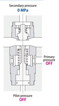
Stop supplying pilot pressure after clamp pressure is released.
