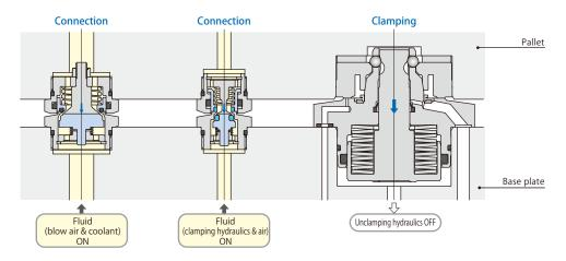
When clamping pallet, coupler connects due to clamp stroke of pallet clamp.
