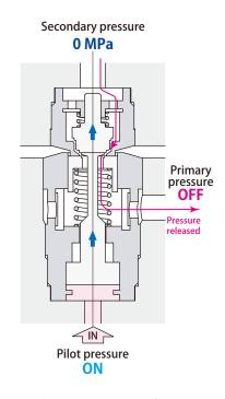
Supply pilot pressure after connection and release the clamp pressure.
