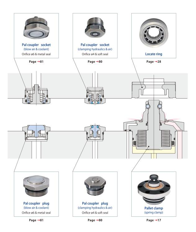
Select one of either spring clamp (model CPC), hydraulic clamp (model CPH) or air clamp (model CPY).
