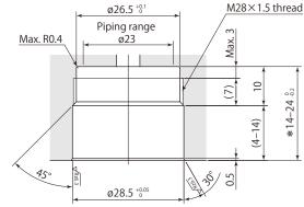
\*: When using Pal fix as a set, be sure to set depth to 24<sub>-02</sub>. Refer to pages →66-77 for details on Pal fix.
