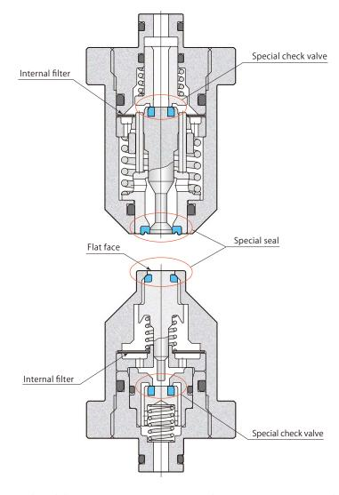
Spill amount (liquid drip amount per connection or disconnection) 0.01 mL or less
