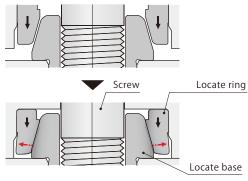
By means of elastic deformation
