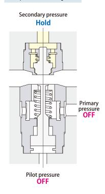
Stop supplying pilot pressure after secondary pressure is built up.
