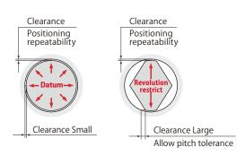
The positioning repeatability spoils when providing a large clearance.
