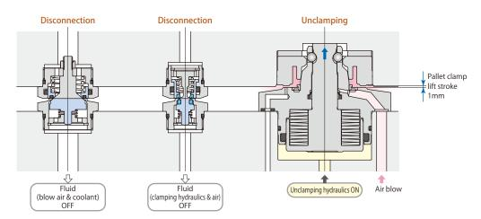
When unclamping pallet, coupler disconnects due to lift stroke of pallet clamp.
