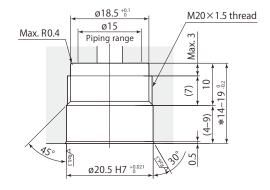
\*:When using Pal fix as a set, be sure to set depth to  $19_{-0.2}^{0}$ . Refer to **pages**  $\rightarrow$ **66–77** for details on Pal fix.
