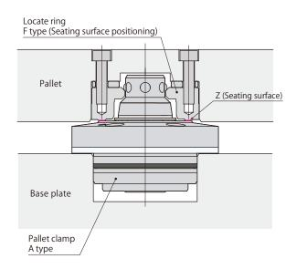
Since Z axis is positioned by 4 points of seating surface with no effect from pitch error, surface accuracy of pallet is sustained at high levels.
