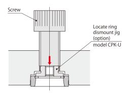
The ring can be removed by a screw.
