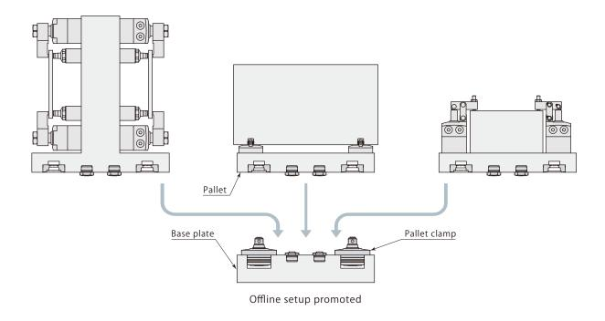
• Implementation of Pal system makes it possible to perform setting of workpiece on jigs of machine table accurately and significantly reduces setup time that was previously necessary for alignment.
