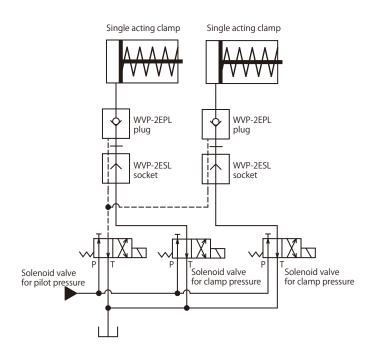
A solenoid valve which switches to Tank port connection except supplying pressure to the circuit should be used to avoid back pressure.
