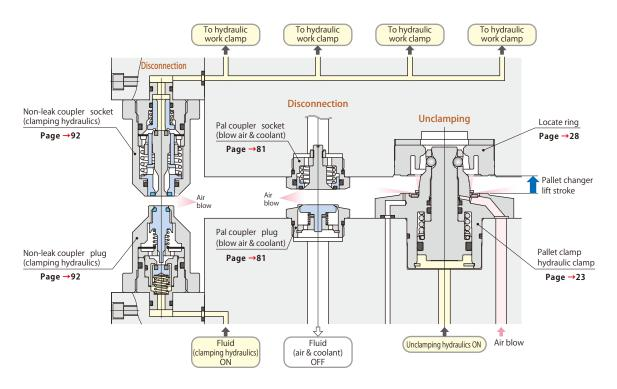
When unclamping pallet, coupler disconnects due to lift stroke of pallet changer, with hydraulics sustained.
