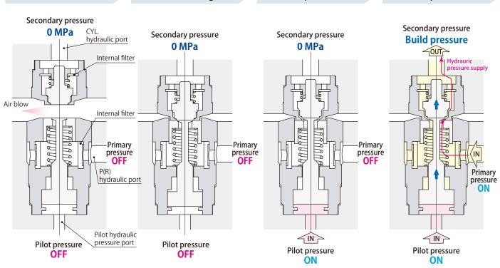
Do not supply primary and pilot pressure when coupler disconnected state.
