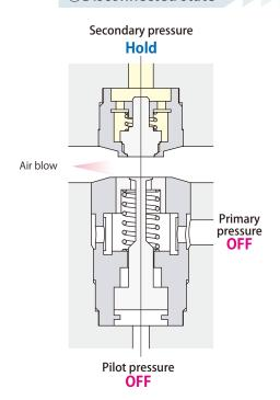
Do not supply primary and pilot pressure when coupler disconnected state.
