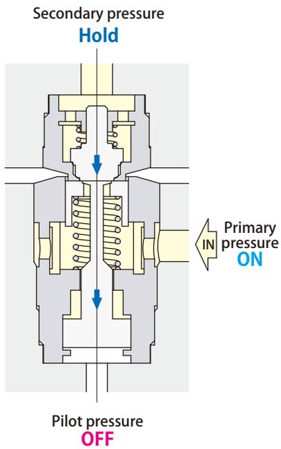
Stop supplying pilot pressure after secondary pressure is built up.
