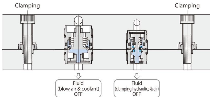
Precise positioning can be made by simply tightening the screws, and couplers can be connected at the same time.
