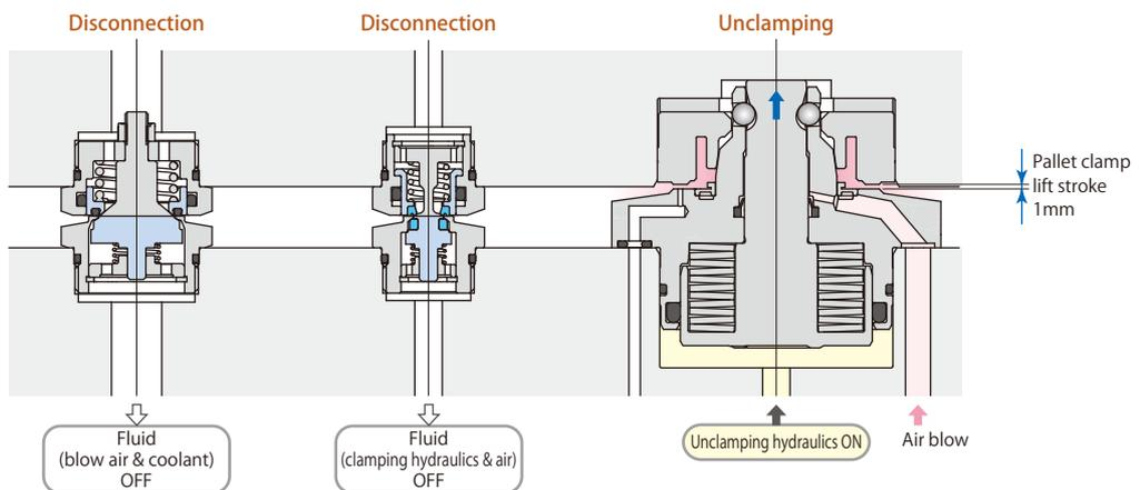
When unclamping pallet, coupler disconnects due to lift stroke of pallet clamp.
