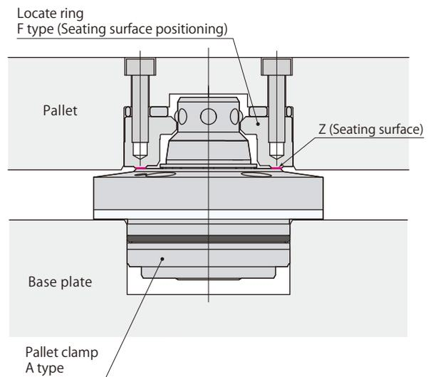
Since Z axis is positioned by 4 points of seating surface with no effect from pitch error, surface accuracy of pallet is sustained at high levels.
