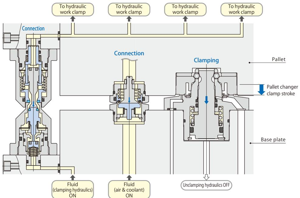
When clamping pallet, coupler connects due to clamp stroke of pallet changer, with hydraulics sustained.
