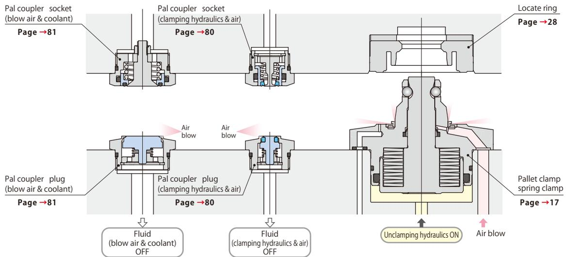
Pallet unclamped and coupler disconnected
