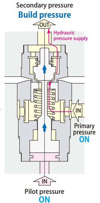
Supply primary pressure after pilot pressure is supplied.
