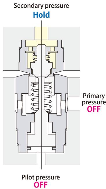
Stop supplying primary pressure after pilot pressure is supplied.
