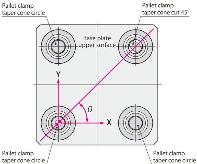
The pitch error between XYZ axes positioning pallet clamp and  $\theta$  Z axes positioning pallet clamp is tolerated by cut type taper cone even under thermal change conditions.
