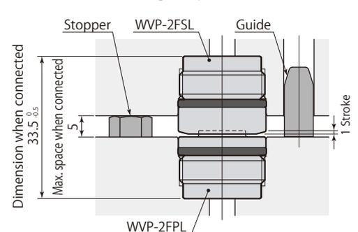
Air & coolant coupler with large orifice area and capability to accommodate large flow rates.
