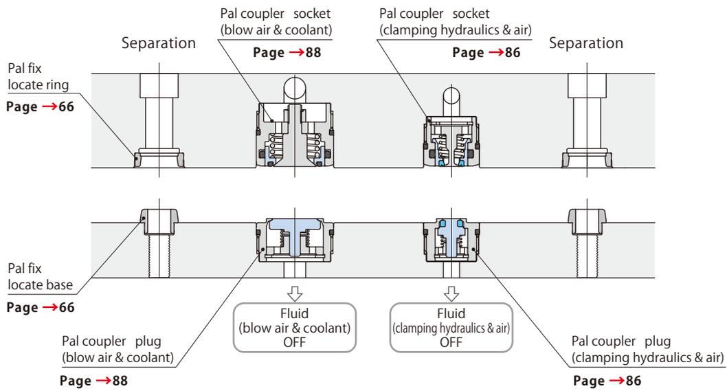
Pallet clamped and coupler connected
