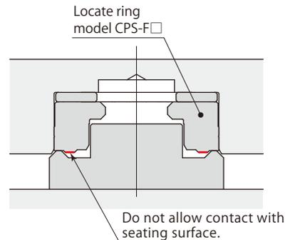
\* : 1mm for CPS-□□F (Locate ring for flange mounting)
