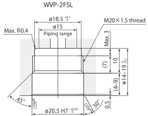
\* :When using Pal fix as a set, be sure to set depth to 19.0. Refer to pages →66-77 for details on Pal fix.
