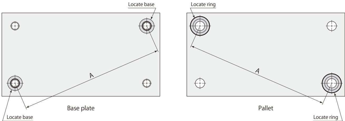
Pitch tolerance of A dimension
