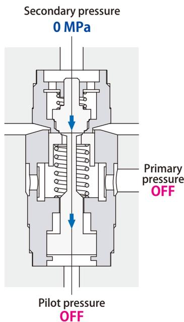
Stop supplying pilot pressure after clamp pressure is released.
