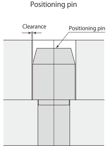
Taper cone makes attaching / detaching easy
