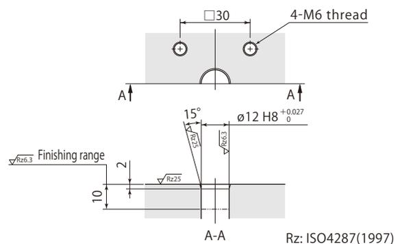
● Perform installation with plug below so metal chips are less likely to adhere and air blowing can be performed properly.
