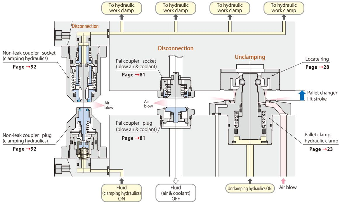
When unclamping pallet, coupler disconnects due to lift stroke of pallet changer, with hydraulics sustained.
