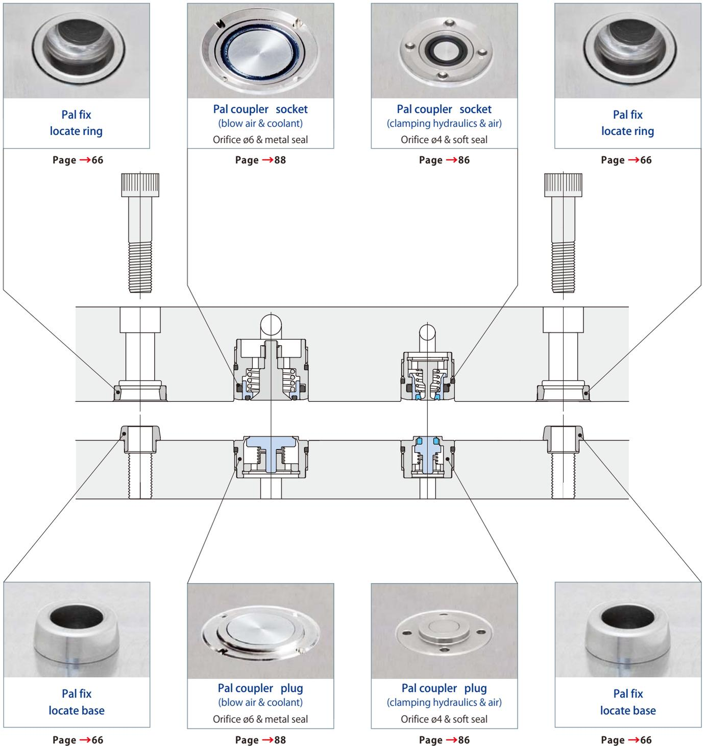
It is a taper cone model with dual surface contact to position high-accuracy.
