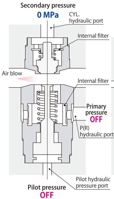
Do not supply primary and pilot pressure when coupler disconnected state.
