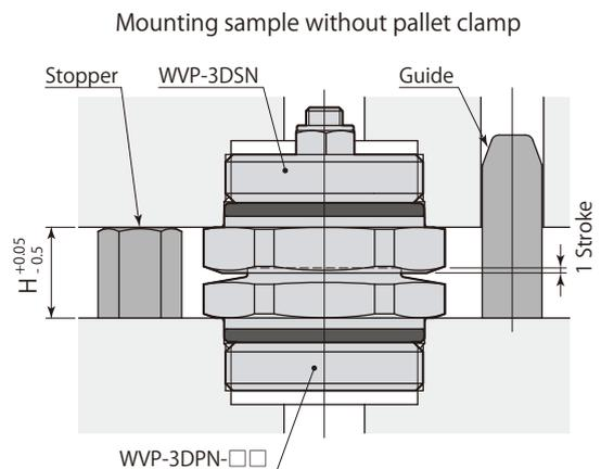
**Hydraulic and air coupler with zero hydraulic oil leak with special seal at tip section**
