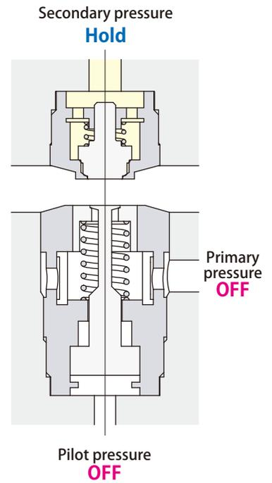
Clamp pressure is kept even after coupler is disconnected.
