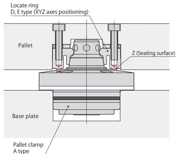
The pitch error between XYZ axes positioning pallet clamp and  $\theta$  Z axes positioning pallet clamp is tolerated by cut type taper cone even under thermal change conditions.
