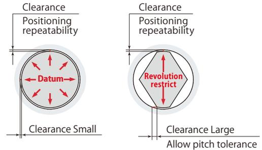
The positioning repeatability spoils when providing a large clearance.
