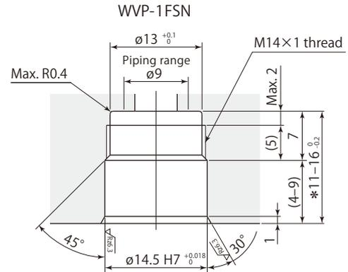
\*: When using Pal fix as a set, be sure to set depth to 16<sup>0</sup><sub>-0.2</sub>. Refer to pages →66-77 for details on Pal fix.
