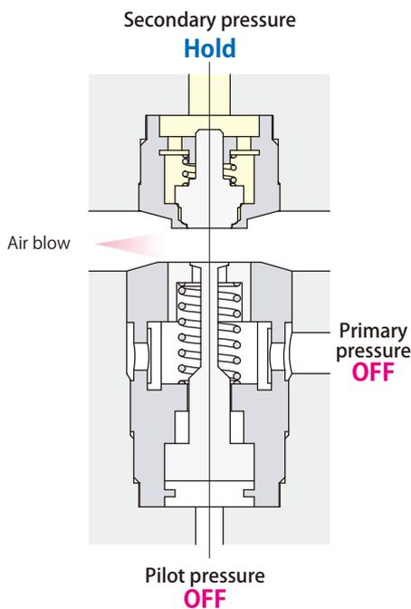
Do not supply primary and pilot pressure when coupler disconnected state.
