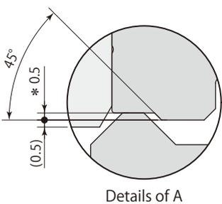
\* : 1mm for CPS-□□F (Locate ring for flange mounting)
