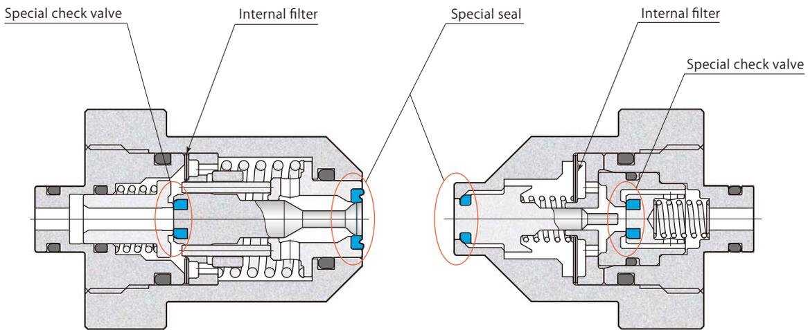
Spill amount (liquid drip amount per connection or disconnection) 0.01 mL or less
