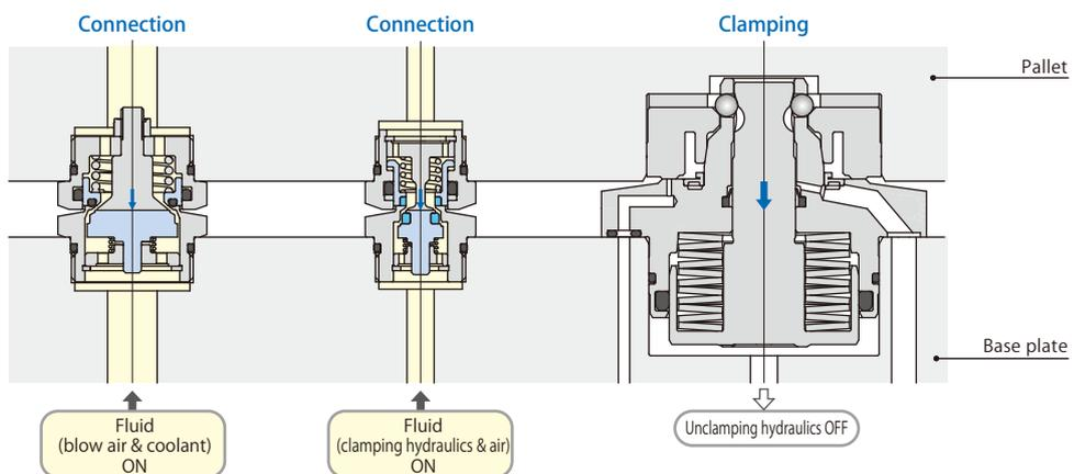
When clamping pallet, coupler connects due to clamp stroke of pallet clamp.
