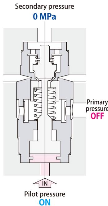
Supply pilot pressure to open the check valve.
