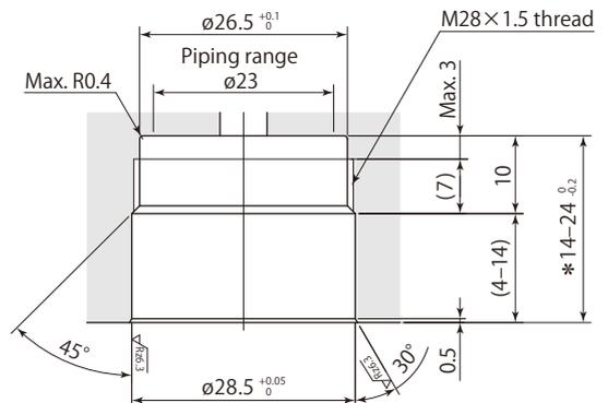
\* : When using Pal fix as a set, be sure to set depth to 24<sub>0.2</sub><sup>0</sup>. Refer to pages →66-77 for details on Pal fix.
