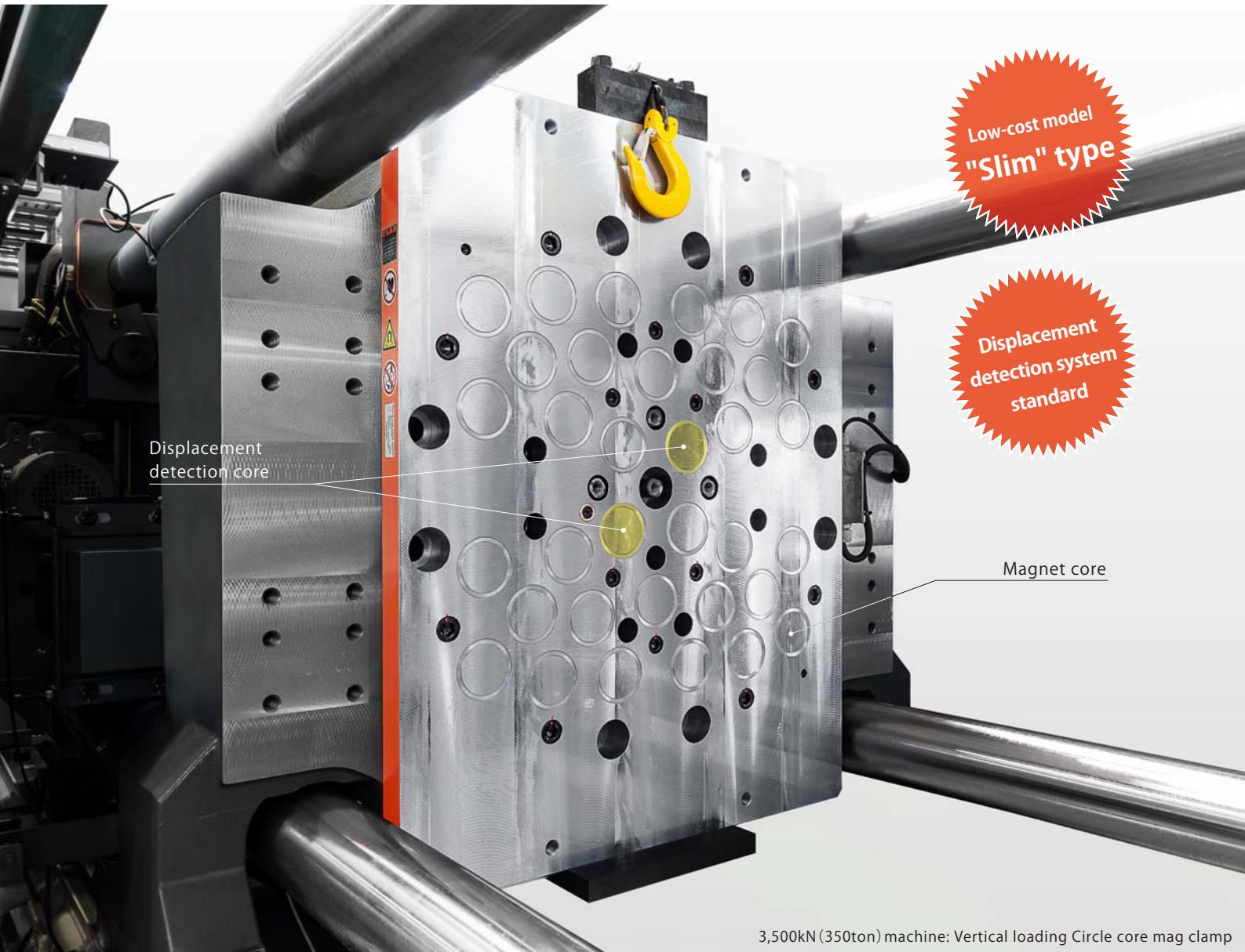
3,500kN (350ton) machine: Vertical loading Circle core mag clamp
