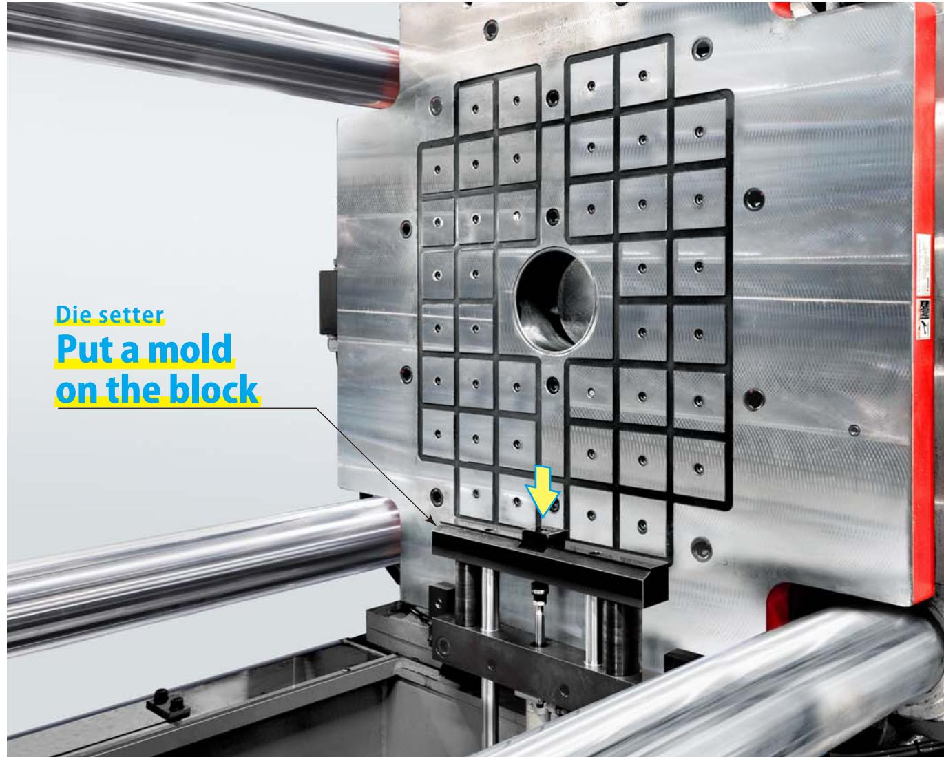
3,500kN (350ton) IMM Vertical loading Die setter & Mag clamp
