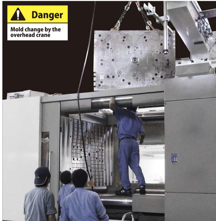
Carelessly coming under the craned mold.
