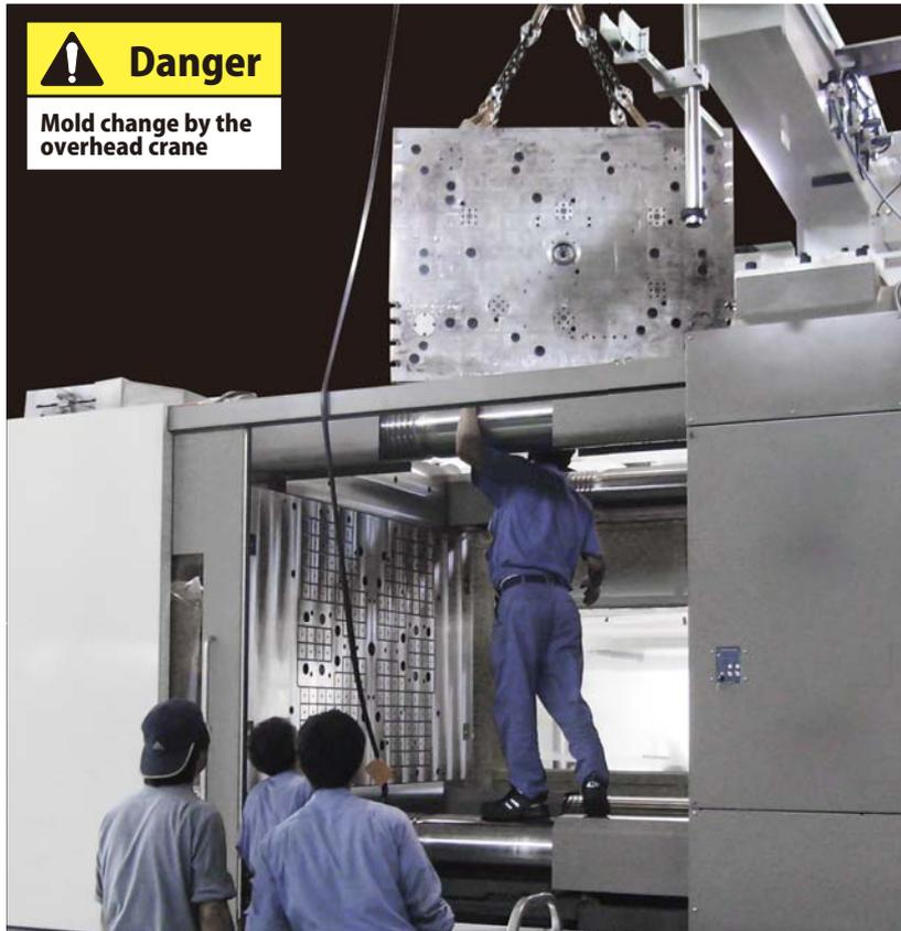
Carelessly coming under the craned mold.
