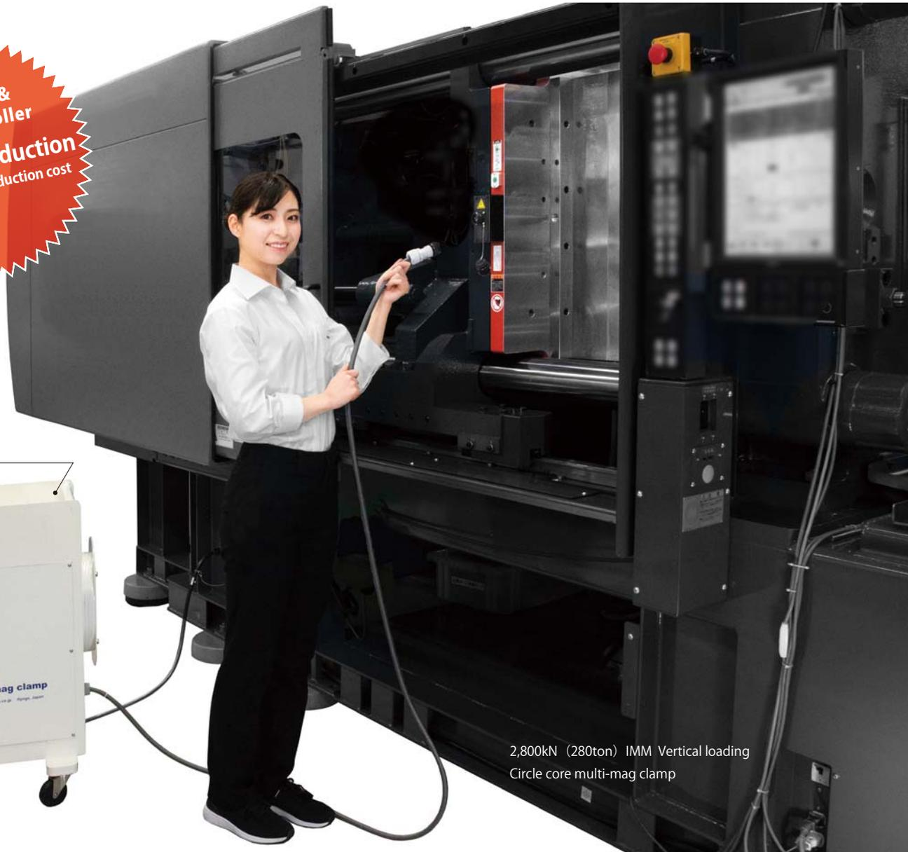
2,800kN (280ton) IMM Vertical loading
