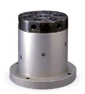
Rotary joint model WRB was developed for low pressure applications. Aluminum is adopted as body material to reduce the weight. This is a center through type, which the through bore of rotary shaft can be used for coolant piping.
