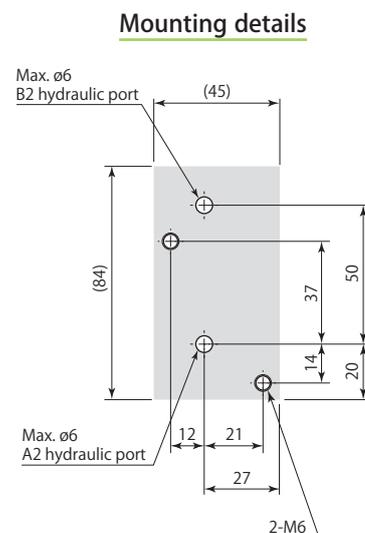
For manifold piping, the mounting surface finish must be no rougher than Rz6.3 (ISO4287:1997).
