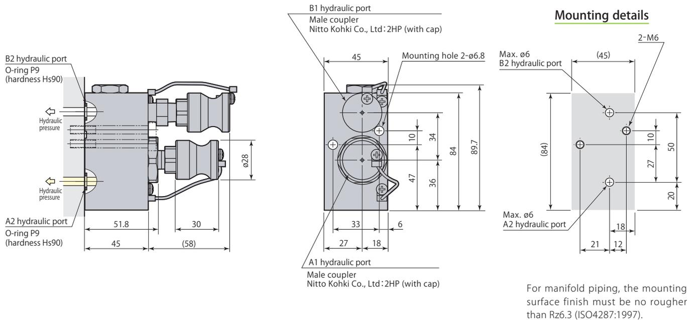
**VCB-LT** Piping mounting \*With internal filter (A1 & A2 hydraulic ports)
