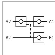
This is a non-leak valve, with which coupling of double acting clamp can be performed easily and clamping circuit pressure can be retained over a long period of time after disengagement of hydraulic pressure source.
