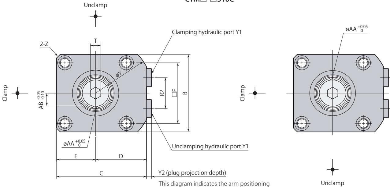
This diagram indicates the arm positioning pin groove at unclamped condition.
