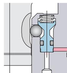
Poppet structure ensures superior sealing performance and can create large differential-pressure when the valve is opening and closing, and air leakage can be minimized.
