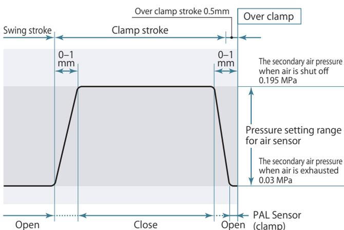
The diagram shown on the left indicates the relation between the PAL sensor, piston stroke, and secondary air pressure. (The pressure shown in the diagram is a reference based on the 0.2 MPa of primary air pressure for one piece of clamp.)
