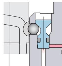
Poppet structure ensures superior sealing performance and can create large differential-pressure when the valve is opening and closing, and air leakage can be minimized.
