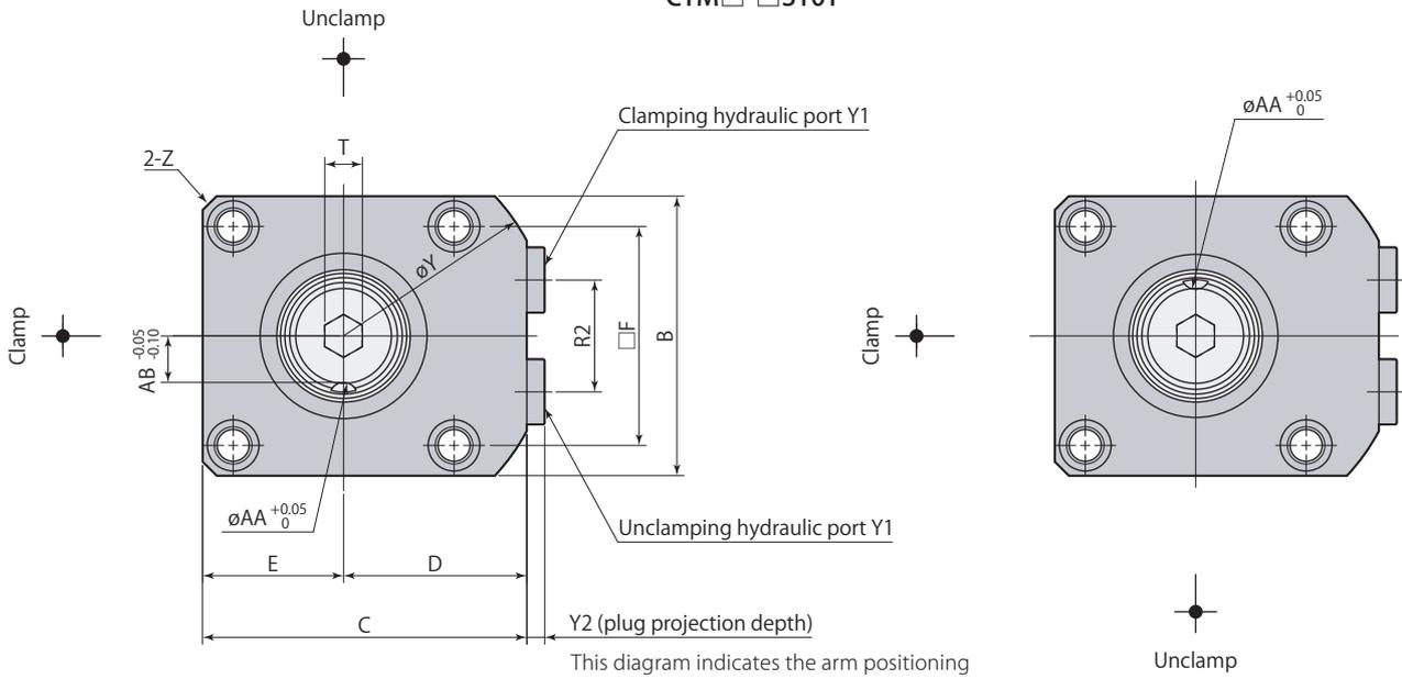
This diagram indicates the arm positioning pin groove at unclamped condition.
