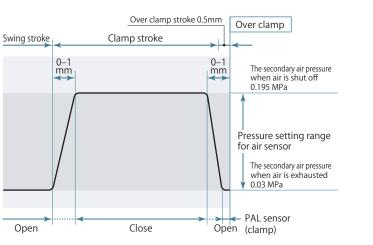
The diagram shown above indicates the relation between the PAL sensor, piston stroke, and secondary air pressure. (The pressure shown in the diagram is a reference based on the 0.2 MPa of primary air pressure for one piece of clamp.)
