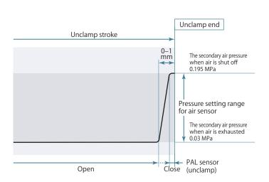
The diagram shown above indicates the relation between the PAL sensor, piston stroke, and secondary air pressure. (The pressure shown in the diagram is a reference based on the 0.2 MPa of primary air pressure for one piece of clamp.) Since the new PAL sensor works with less air-leakage compared to previous sensor valve,
