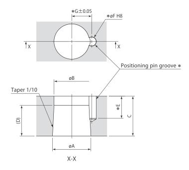
\*: No need to machine the pin groove (E, øF, G) unless positioning pin is used for the arm.
