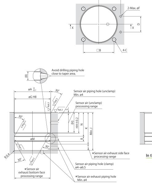
\*: Sensor air exhaust piping hole must be made on
