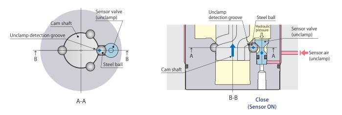
The steel ball seats in the unclamp detection groove when the cam shaft reaches unclamp end, and a sensor valve (unclamp) is pushed down to shut off the sensor air by hydraulic force, and detects the unclamped condition.
