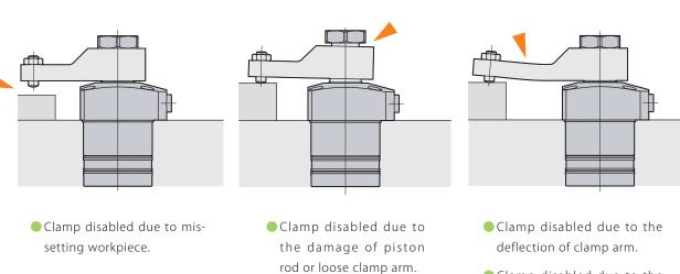
Clamp disabled due to the abrasion on the tip of clamp arm during prolonged use.
