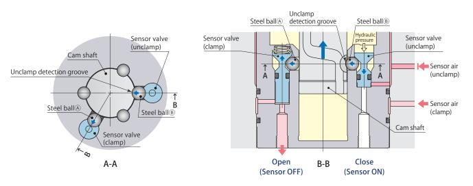
• The steel ball <sup>®</sup> seats in the unclamp detection groove when the cam shaft reaches unclamp end, and a sensor valve (unclamp) is pushed down to shut off the sensor air by hydraulic force. The sensor valve (clamp) is pushed up by the steel ball <sup>®</sup> to open for air exhaust and detects the unclamped condition.
