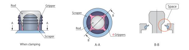
Because of space between scraper, gripper and the rod, air blow must always be performed to prevent intrusion of chips.
