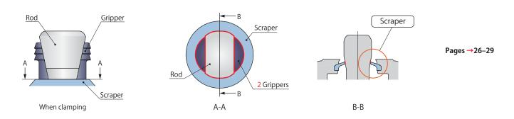
Because there is no space between scraper, gripper and the rod, it is not necessary to perform air blow during cutting process.
