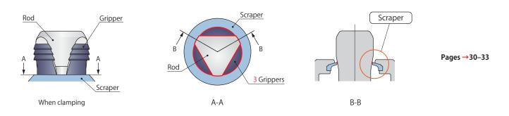
Because there is no space between scraper, gripper and the rod, it is not necessary to perform air blow during cutting process.
