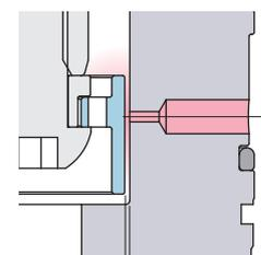
Air leaks easily due to a large space.
