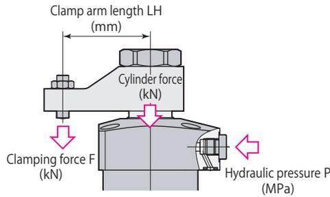
Clamping force varies depending on the clamp arm length (LH) and hydraulic pressure (P).
