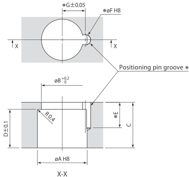
\* : No need to machine the pin groove (E,  $\phi F$ , G) unless positioning pin is used for the arm.
