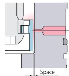
Air leaks easily due to a large space.
