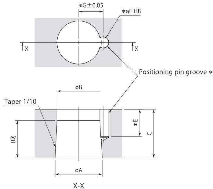
\*: No need to machine the pin groove (E,  $\phi F$ , G) unless positioning pin is used for the arm.
