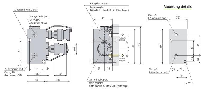
For manifold piping, the mounting surface finish must be no rougher than Rz6.3 (ISO4287:1997).
