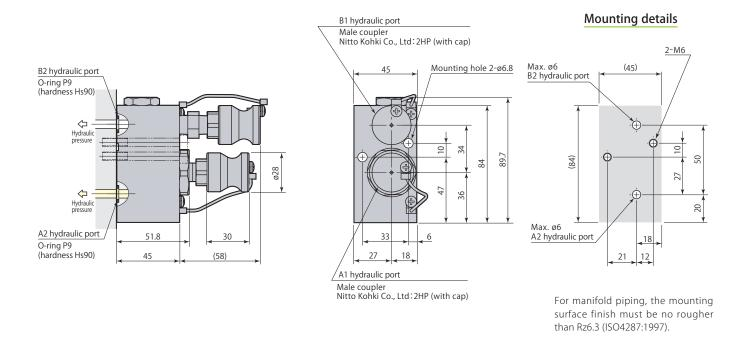
VCB-HT Piping mounting \*With internal filter (A1 & A2 hydraulic ports)
