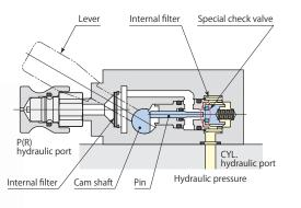
This is a non-leak valve, with which coupling of single acting clamp can be performed easily and clamping circuit pressure can be retained over a long period of time after disengagement of hydraulic pressure source.
