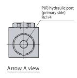
**VRG-** VHD linking \*With internal filter (P & CYL. hydraulic ports)
