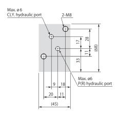
For manifold piping, the mounting surface finish must be no rougher than Rz6.3 (ISO4287:1997).
