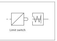
Detects a condition of hydraulic pressure (ON or OFF) in the clamp circuit. If you install a limit switch, you can have an interlock protection device (such as stopping the machining) against pressure OFF condition.
