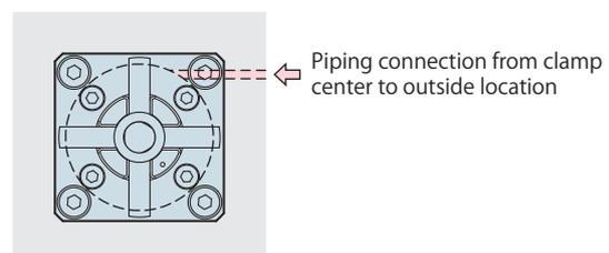
For the double-action gasket piping expansion clamp — model CGS-N2, the piping connection port location will differ depending on the clamp mounting angle. Thus, piping hole layout becomes complicated and jig production and design will be difficult. (Figure 2-b)
