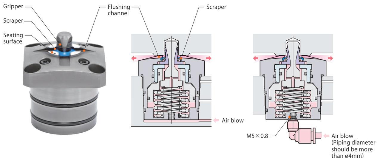
Jig design and production made easy with cartridge piping.
