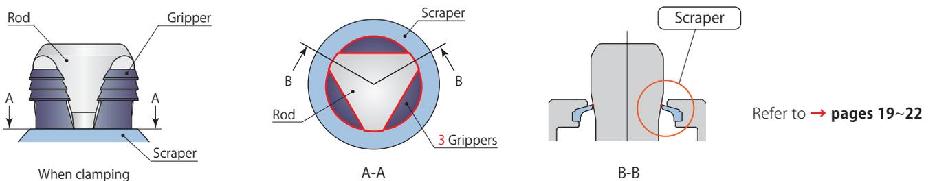
Because there is no space between scraper, gripper and the rod, it is not necessary to perform air blow during cutting process.
