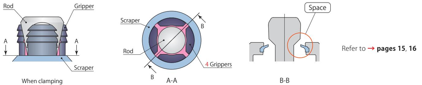
Because of space between scraper, gripper and the rod, air blow must always be performed to prevent intrusion of chips.
