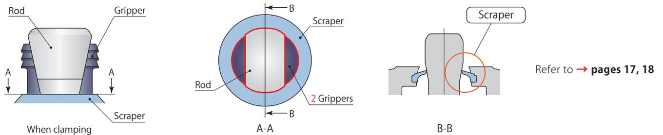
Because there is no space between scraper, gripper and the rod, it is not necessary to perform air blow during cutting process.
