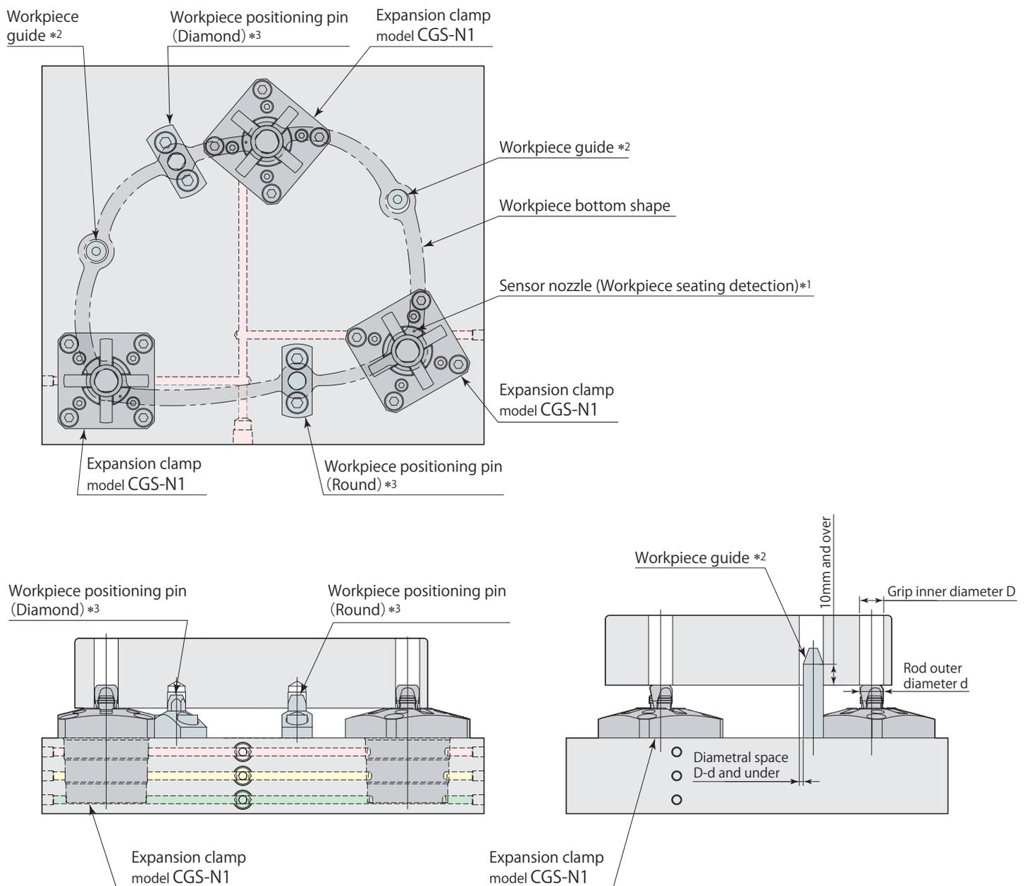
\*1 : The sensor nozzle (workpiece seating detection) can be set at any position by installation phase of CGS and can be friend to the rib shape of workpiece bottom. As the internal design can be made easily, piping layout is not required to change according to installation phase of CGS, the jig.
