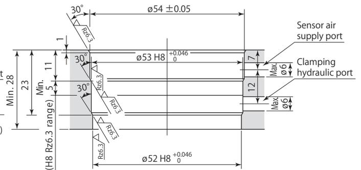
\*: Blow air supply port (sensor air exhaust port) must be provided on either side or bottom face.
