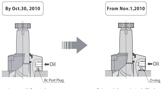
Plug the o-ring port with Rc port plug after removing the o-ring and G port plug. (Rc port plugs are packed with the clamp) O-ring seals the port instead of Rc plug. Do not remove the o-ring initially mounted with the clamp.
