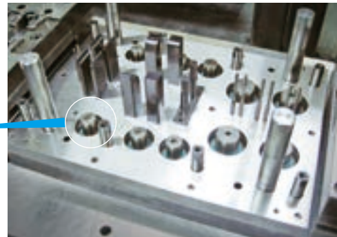
4,000kN (400tonf) Progressive press lower Mini N2 gas spring adopted example
