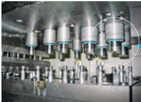
4,000kN (400tonf) Progressive press upper Mini N2 gas spring adopted example
