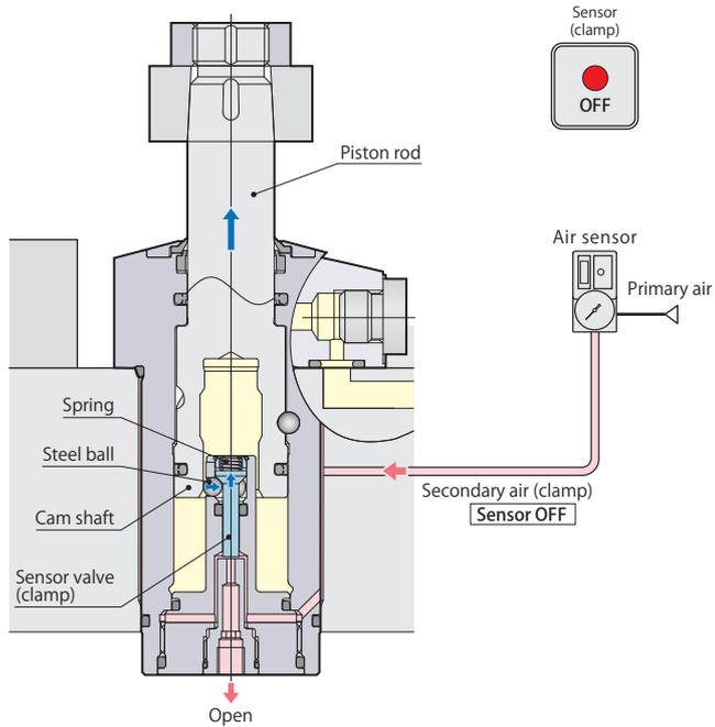
Sensor signal (clamp) **OFF** Unclamp
