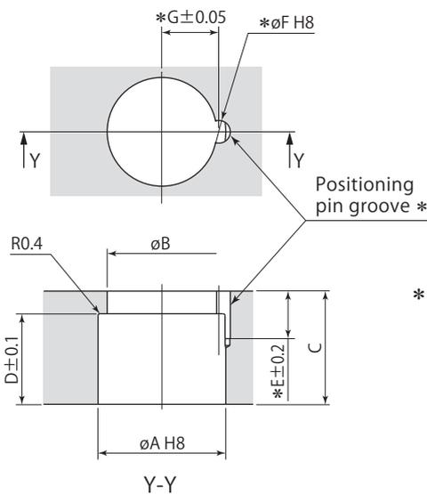
\* : No need to machine the pin groove (E,  $\phi F$ , G) unless positioning pin is used for the arm. The positioning pin enables a clamp arm to locate on the clamp firmly and easily.
