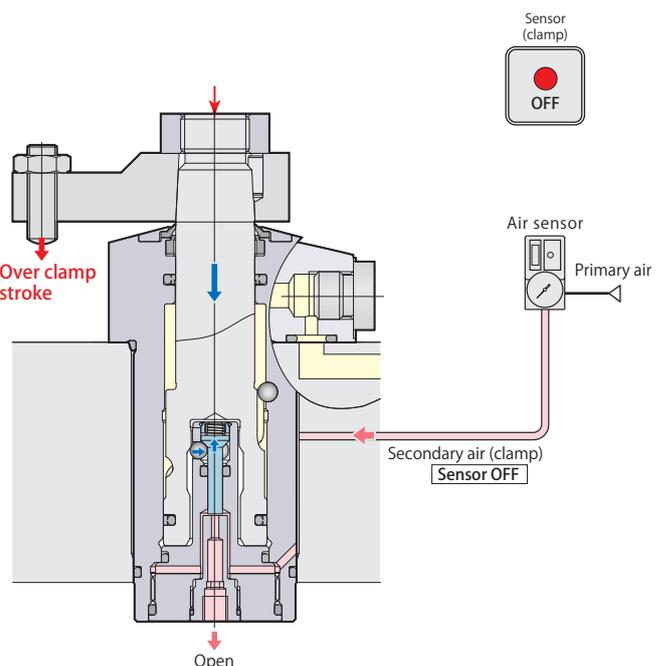
Sensor signal (clamp) **OFF** Over clamp stroke (Incomplete clamp)
