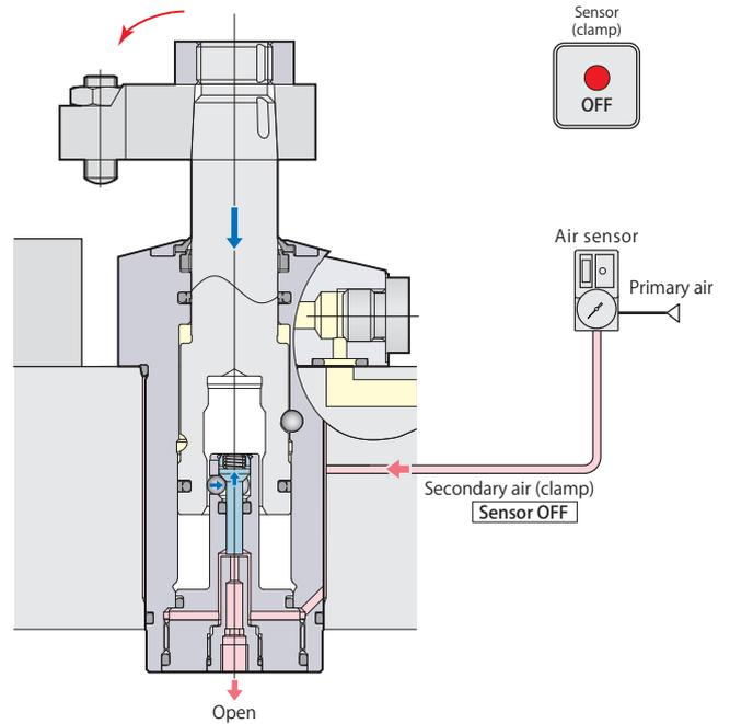
Sensor signal (clamp) **OFF** In the middle of swing stroke
