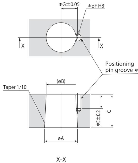
\* :No need to machine the pin groove (E,  $\phi F$ , G) unless positioning pin is used for the arm.
