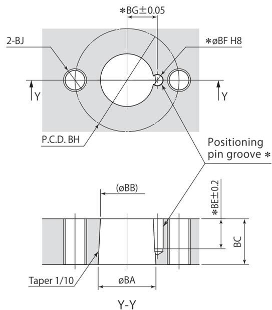
\*: No need to machine the pin groove (BE, øBF, BG) unless positioning pin is used for the arm.
