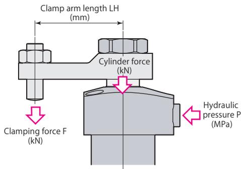
Clamping force varies depending on the clamp arm length (LH) and hydraulic pressure (P).
