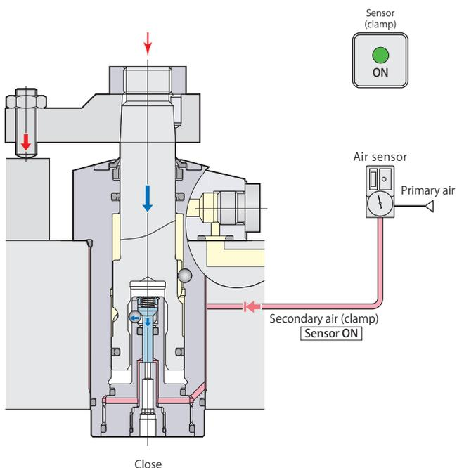
Sensor signal (clamp) **ON** Clamp
