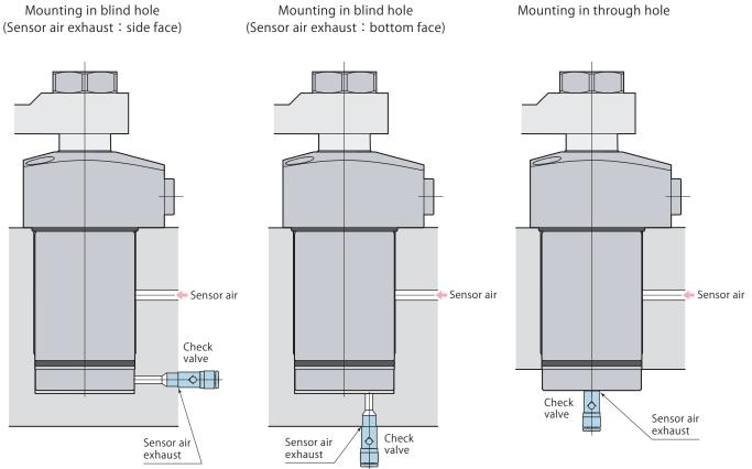
• Use a check valve with cracking pressure of 0.005 MPa or less if there is a risk of metal chips or coolant intrusion. Recommended check valve : AKH or AKB series manufactured by SMC.
