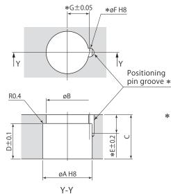
\*:No need to machine the pin groove (E, ØF, G) unless positioning pin is used for the arm. The positioning pin enables a clamp arm to locate on the clamp firmly and easily.
