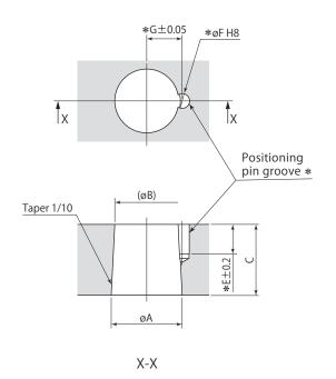
\*: No need to machine the pin groove (E, øF, G) unless positioning pin is used for the arm.The positioning pin enables a clamp arm to locate on the clamp firmly and easily.
