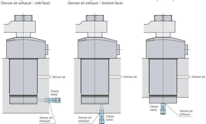
• Use a check valve with cracking pressure of 0.005 MPa or less if there is a risk of metal chips or coolant intrusion. Recommended check valve : AKH or AKB series manufactured by SMC.
