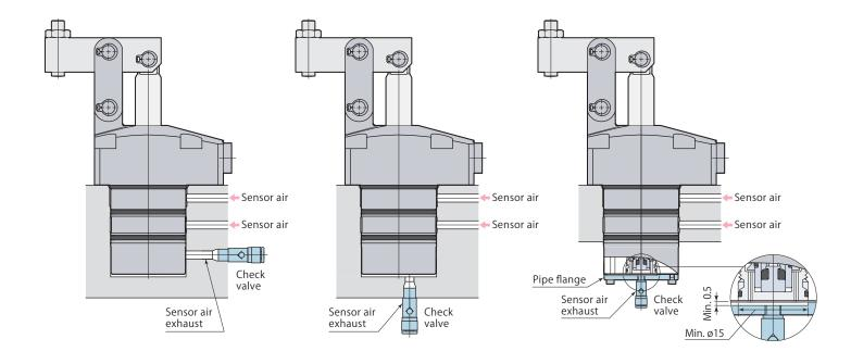
• Use a check valve with cracking pressure of 0.005 MPa or less if there is a risk of metal chips or coolant intrusion. Recommended check valve : AKH or AKB series manufactured by SMC.
