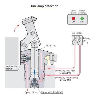
The sensor may not work correctly when the cylinder is not pressurized by hydraulic force because the piston of the clamp moves under such environment. Keep supplying hydraulic force the cylinder all the times.
