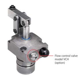
In case of mounting flow control valve model VCH on the G port of the clamp, air bleeding valve should be installed in the piping to the clamp. (VCE Mounting details. Refer to page →78) 7.0
