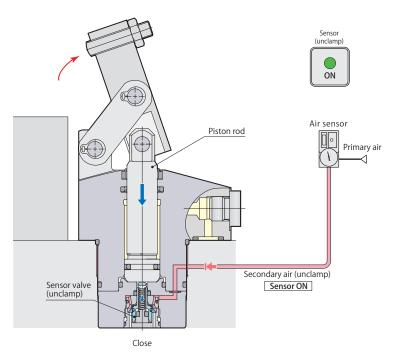
The sensor may not work correctly when the cylinder is not pressurized by hydraulic force because the piston of the clamp moves under such environment. Keep supplying hydraulic force the cylinder all the times.
