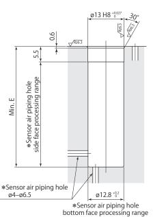
\*: Sensor air piping hole must be made on either side or bottom face.
