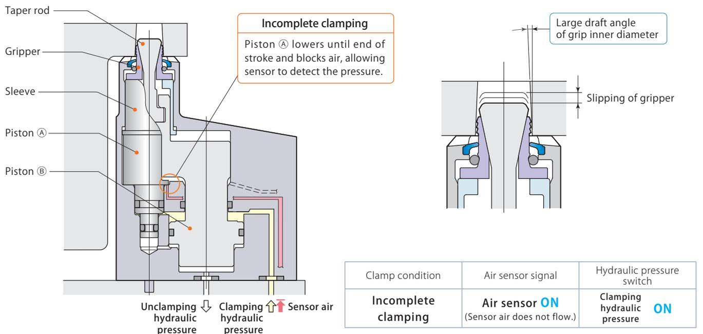
With the development of the non-constant air blow expansion clamp, air consumption will be significantly decreased. The traditional model ordinarily requires 50L/min (0.3MPa) flow rate (when grip inner diameter is  $\varnothing 12$ ). The new model can reduce
