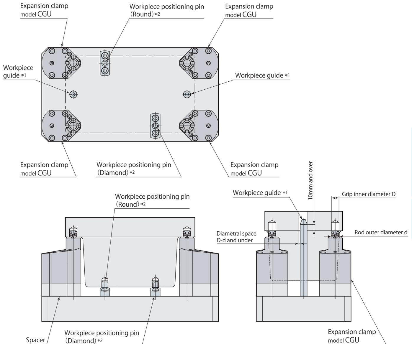
\*1: When using automatic or robotic conveyers, prevent damage to clamp caused from impact by setting workpiece guides. Using the above guide as reference, accurately position the holes when using workpiece guides.
