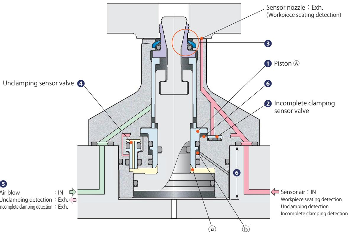
**1 Gripper support mechanism (PAT.)**
