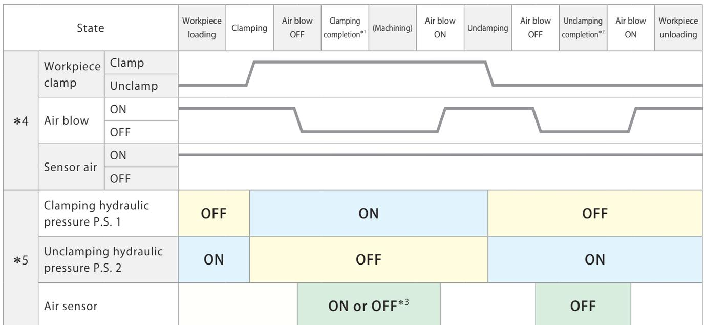
\*1 : Clamping completion : P.S. 1=ON P.S. 2=OFF Air sensor=ON
