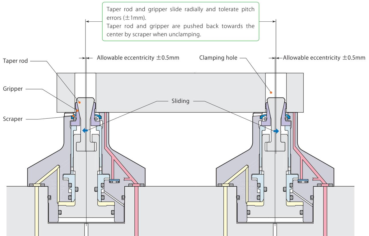
By the eccentric mechanism, the expansion clamp does not have a workpiece positioning function.
