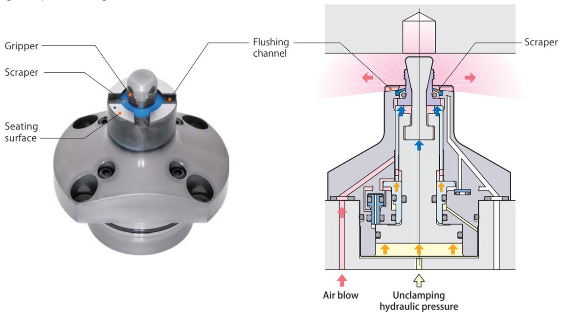
Sensor nozzle detects faulty seating of workpiece
