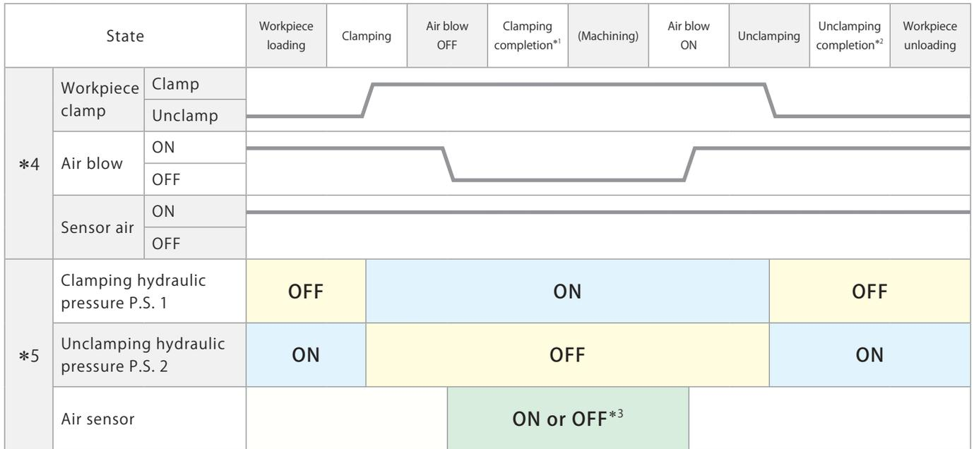
\*1 : Clamping completion : P.S. 1=ON P.S. 2=OFF Air sensor=ON
