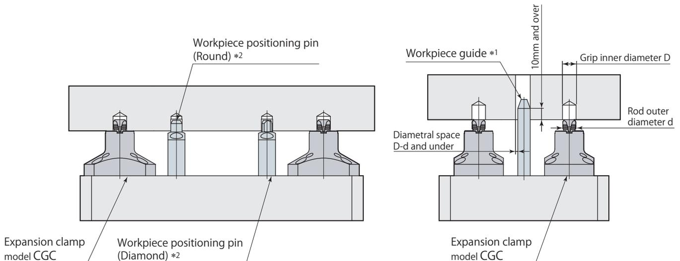
\*1: When using automatic or robotic conveyers, prevent damage to clamp caused from impact by setting workpiece guides. Using the above guide as reference, accurately position the holes when using workpiece guides.
