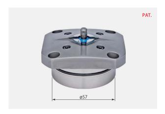
Model CGX-N22- with grip inner diameter ø6~ø8: During clamping, a space is created between the rod, gripper, and scraper as a result of having a small diameter. Constant air blow will be necessary to prevent intrusion of metal chips during the cutting process and during clamping and unclamping.
