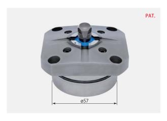
Model CGX-N22E with grip inner diameter ø11~ø13: During clamping, rod will stroke and expand scraper. Thanks to a new mechanism, open space is removed between rod, gripper, and scraper. As chip intrusion is prevented, air blow during cutting process has been eliminated. (Air blow will only be necessary during clamping and unclamping operation.) As a result, air consumption has been significantly reduced compared to the traditional model.
