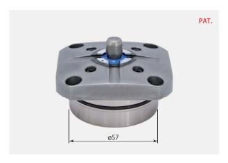
Model CGX-N22E with grip inner diameter ø9 and ø10: During clamping, rod will stroke and expand scraper. Thanks to a new mechanism, open space is removed between rod, gripper, and scraper. As chip intrusion is prevented, air blow during cutting process has been eliminated. (Air blow will only be necessary during clamping and unclamping operation.) As a result, air consumption has been significantly reduced compared to the traditional model.
